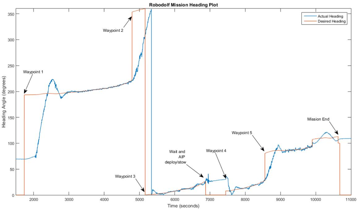
Figure 24: PID controlled heading during mission run.
