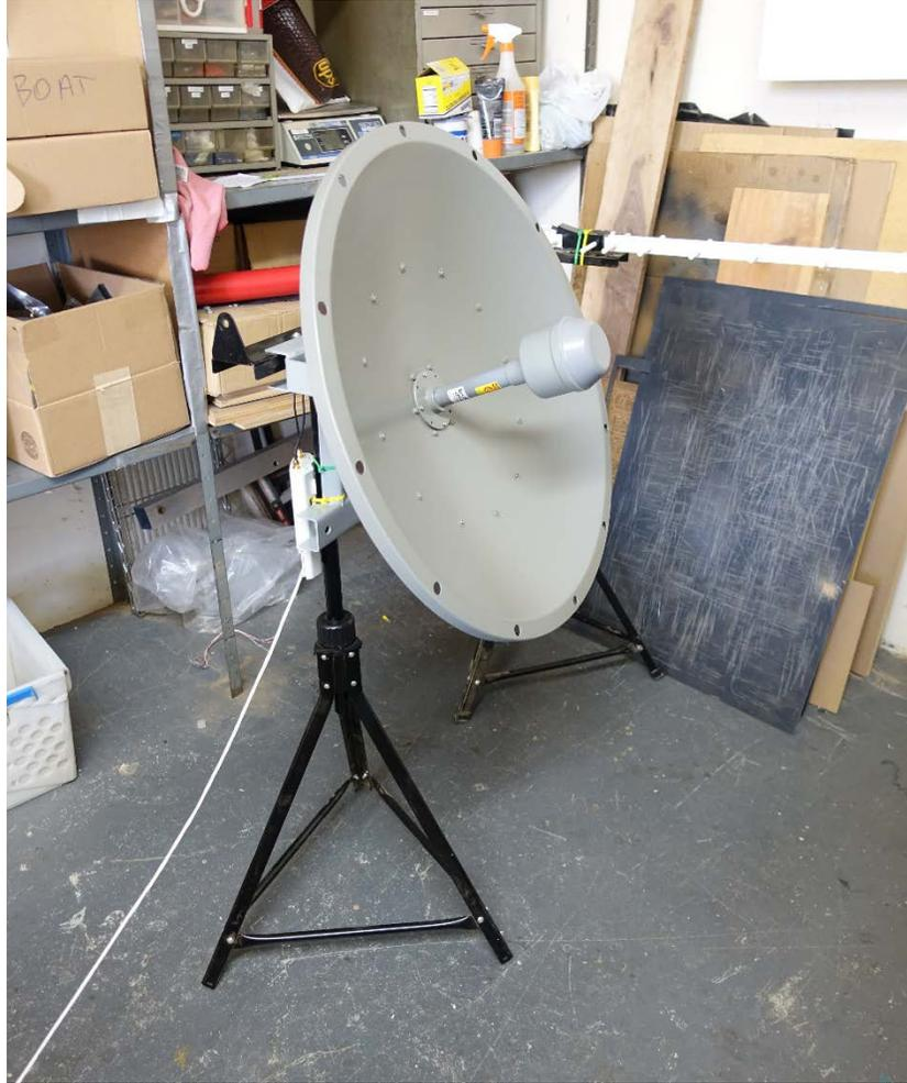
*Figure 14: HSR Shore 2.4 GHz 22 dBi Dual Polarity MIMO Dish Antenna*
