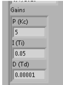
Figure 22: Gains that were selected during Field Test 1 following experimentation.
