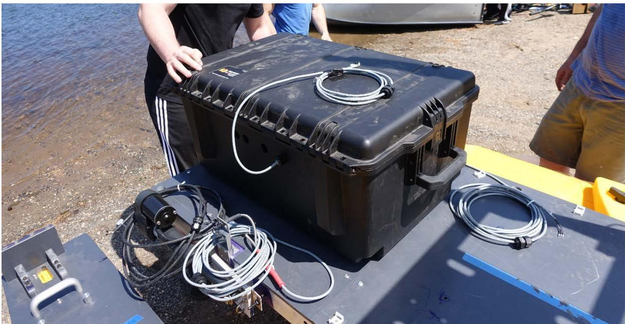
Figure 5: Battery box mounted at the stern. This was very heavy at 100 pounds and required multiple people to lift it in place.
