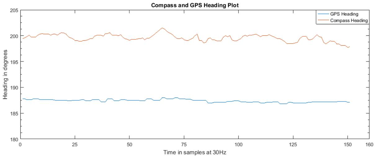
Figure 16: GPS Heading vs Magnetic Compass Heading showing magnetic declination.
