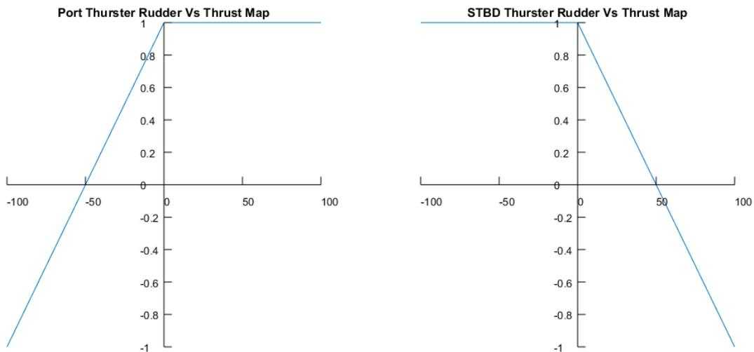
Figure 20: Thrust mapping functions used in Field Test 1. X axis is rudder and Y is thrust. X axis: -100 is full to port, 100 full to STBD. Y axis: 1 is all ahead and -1 is all astern.
