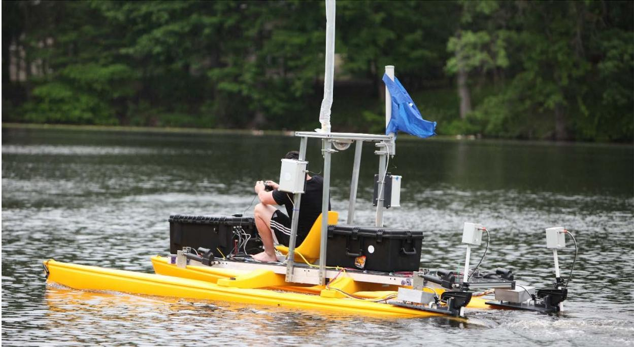
Figure 9: Stern heavy trim with initial configuration. This will be fixed by moving the battery box forward.
