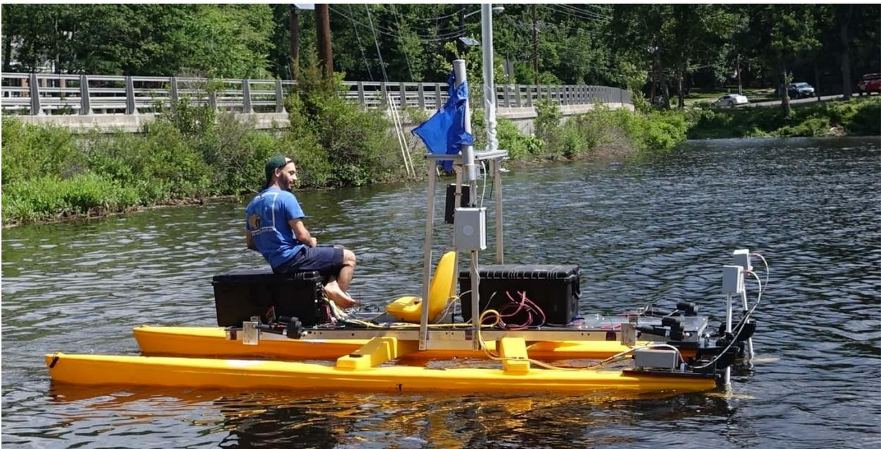
Figure 10: Trim was improved during the field test by shifting the weight of the operator forward.
