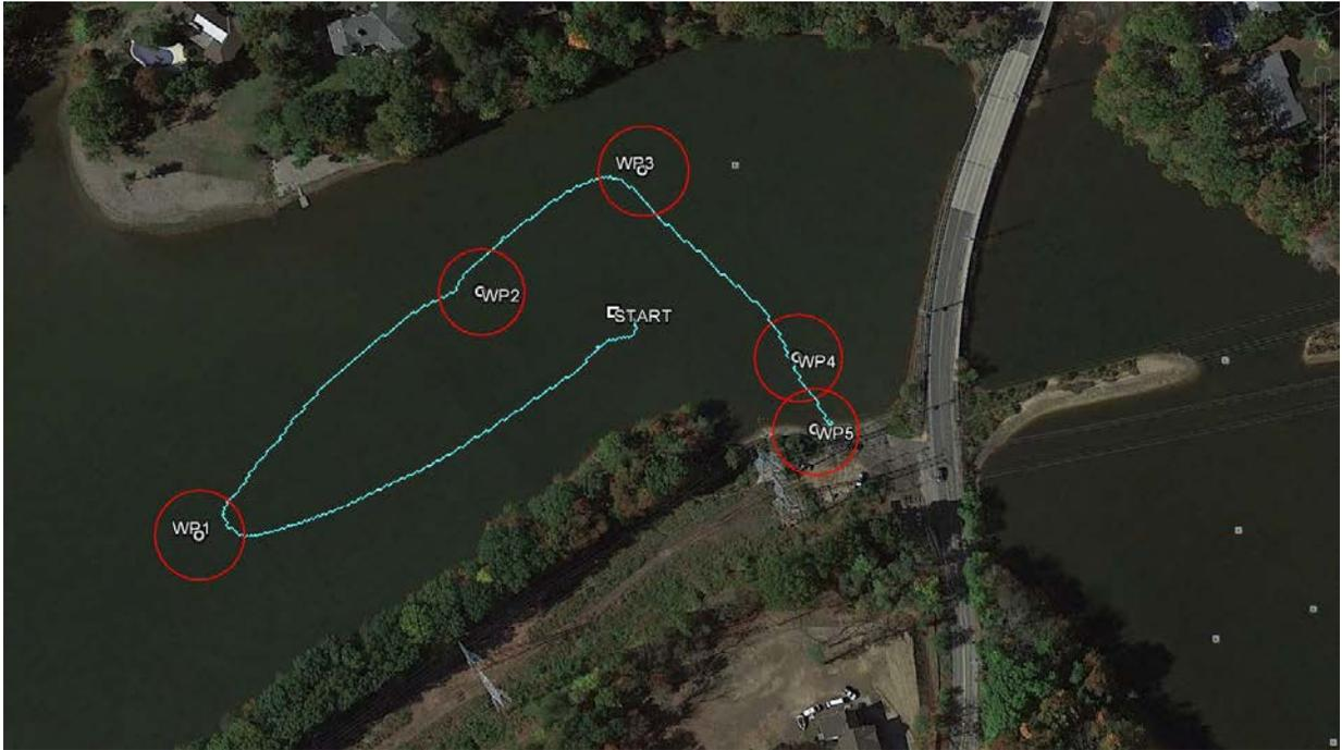
Figure 25: RoboDolf Mission script track. The circles indicate waypoints with a maximum radius of 15 meters.
