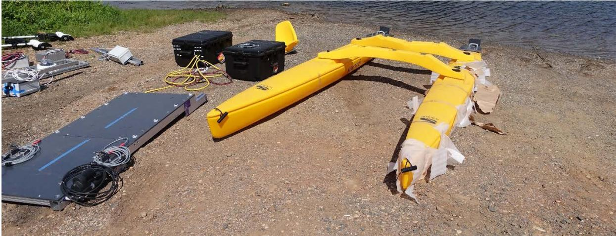
Figure 4: Basic sea-cycle hull assembled and ready for the M-Platform (gray platform on left).
