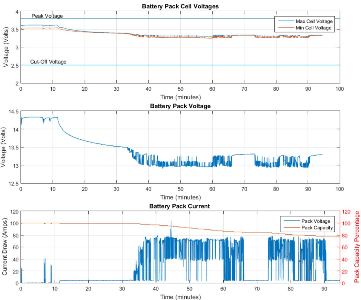
Figure 17: Plot showing the pack information throughout a long run. The fluctuations in the current draw is due to changing throttle commands.
