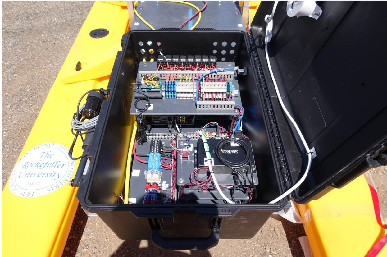
Figure 6: Manual wiring of the main computer box to all other peripheral systems.
