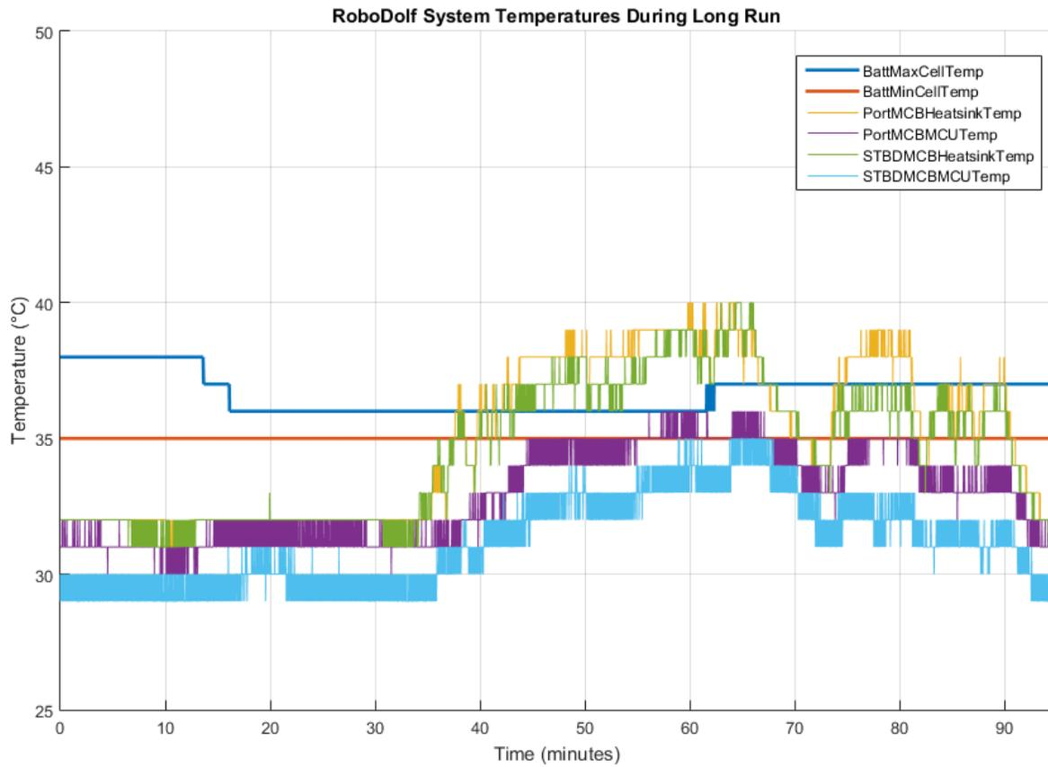
Figure 19: Temperature information from the various temperature sensors onboard the RoboDolf.
