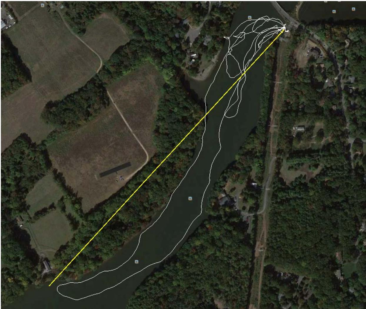
Figure 13: The white shows the track of the longest run done by the RoboDolf. Yellow is the straight line distance of 0.6 miles.
