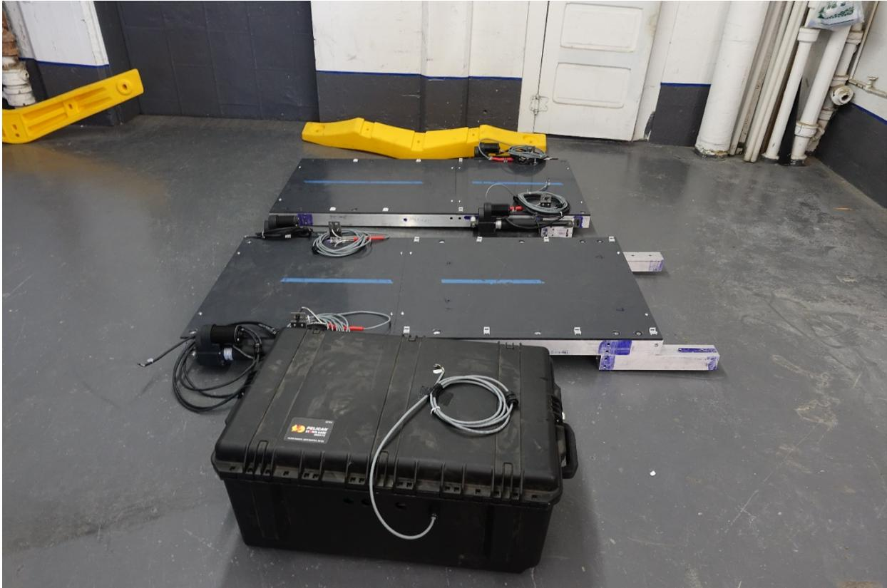
Figure 1: Top to bottom: Forward M-Platform section, Aft M-Platform section, and battery box.
