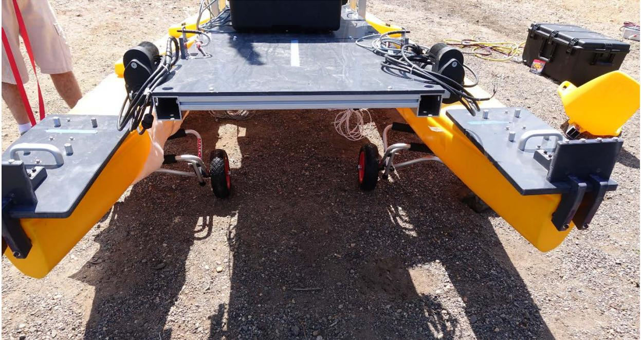
Figure 7: Two kayak dollies, one per hull were used to launch the RoboDolf. They were mounted to the stern and strapped down.
