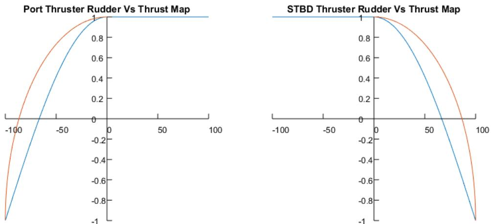
Figure 21: Non-linear thrust mapping which is aimed to give better handling during operator remote control.
